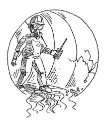
Many construction site situations may pose a "confined space" hazard for which you must monitor the air.
