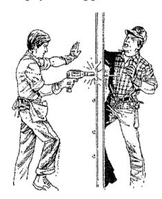
Driving into materials easily penetrated must be avoided unless materials are backed by a substance that will prevent the nail from passing completely through and creating a flying missile hazard on the other side.
