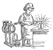
Use of fuel gas—Before a regulator to cylinder valve is connected, the valve must be cracked (opened slightly and closed immediately). This clears the valve of dust or dirt that could enter the regulator.
